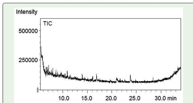
**Figure 1:** Total ion chromatography of ethyl acetate. The ethyl acetate was the solvent control. The total ion chromatography of ethyl acetate was obtained under the GC-MS Conditions. Temperature programmed gas chromatography and electron impact (EI) ion source were used for the analysis of complex samples that we described in the methods.
