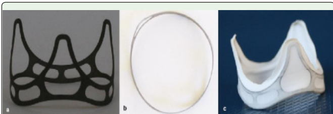
Figure 2: a) Titanium stent, b) titanium stent from above showing the thin thickness and c) titanium stent covered with PTFE using the encapsulation technology.
