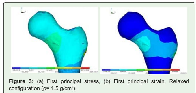
**Figure 3:** (a) First principal stress, (b) First principal strain, Relaxed configuration (ρ= 1.5 g/cm<sup>3</sup>).
